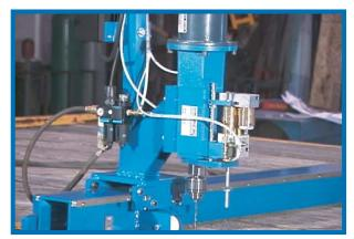
The powerful drill unit adds precision to deck drilling. The job is completed faster and more accurately and broken and dulled tooling is greatly reduced
