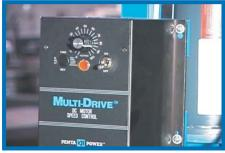
Optional 3/4 hp DC spindle motor can be varied from 0 to 1700 rpm.
