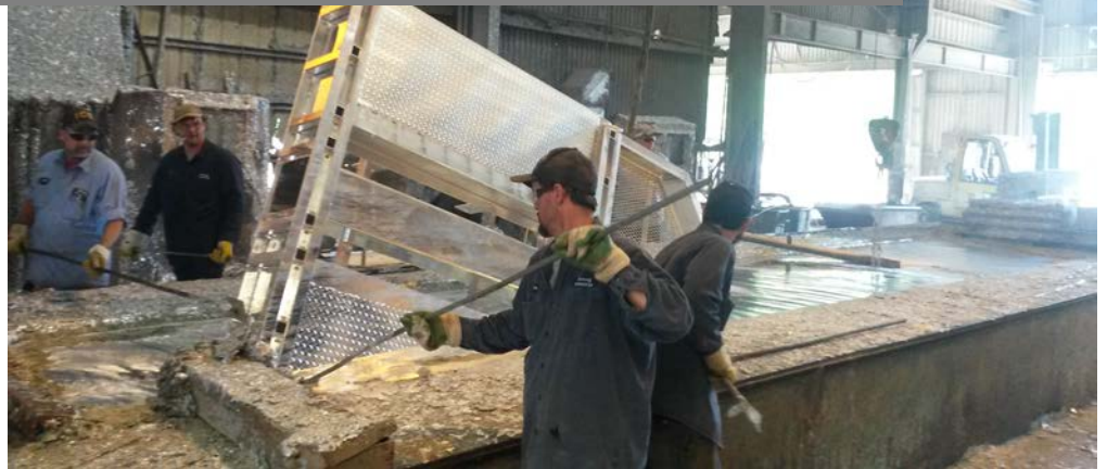
As it is removed, workers skim floating dross out of the way.
