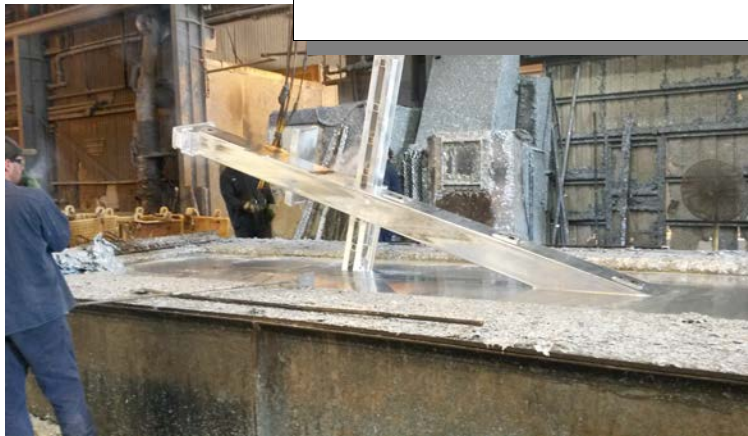
As it is removed, workers skim floating dross out of the way.
