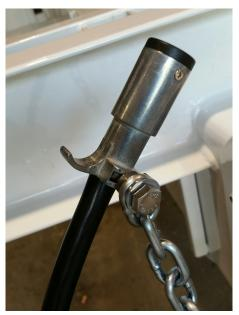
A Mize TC6M-X Trailer End Commector Accepts a bolt to use to attach the chain.
