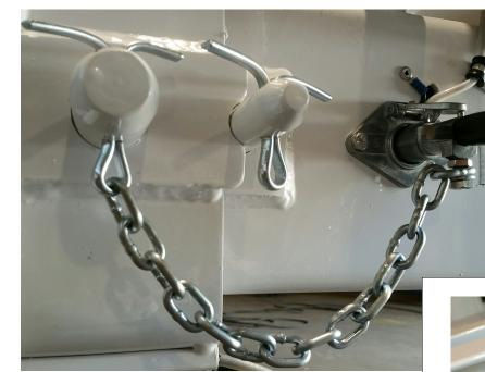
In 2015 the system for ensuring operators unplug the electrical connection before extending or retracting the trailer tongue was enhanced.
