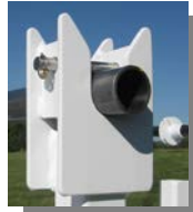
Funnel shaped Spindle Catch.
